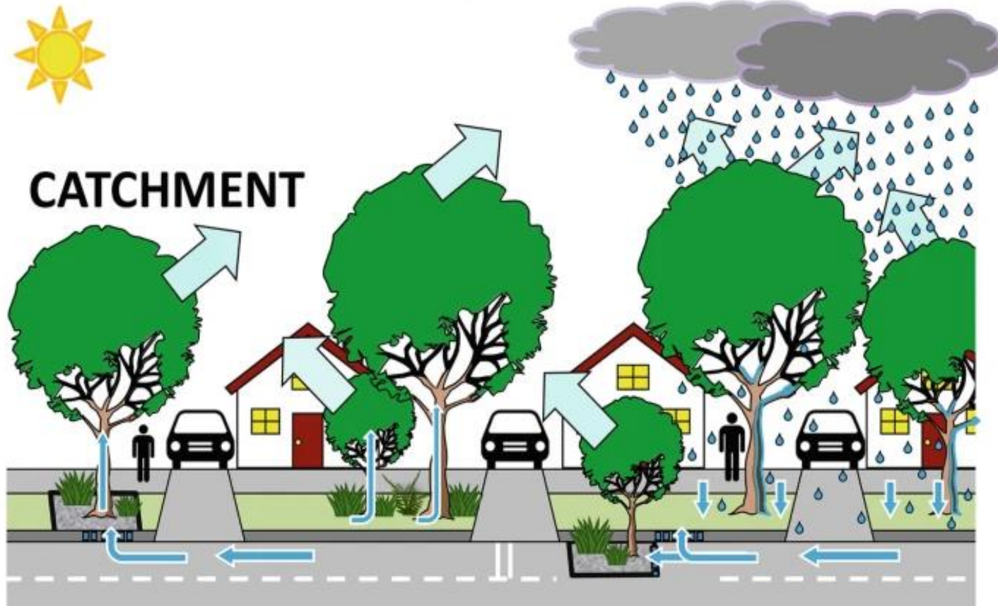
Figure 4. Partitioning of precipitation fluxes in urban trees. Retrieved from (Reyes, 2016).
